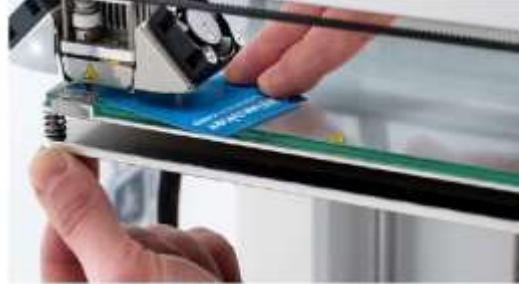
Prepare your plate for the perfect 1st layer by following your 3D printers bed calibration method (make sure to do it properly and maybe even 2 times)
