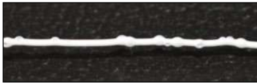
Example of a very 'wet' filament with moisture bubbles after extrusion
