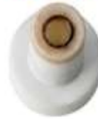
Check your PTFE (if your printer has this in the hotend) for problems. (Brown / Crunchy = bad)
