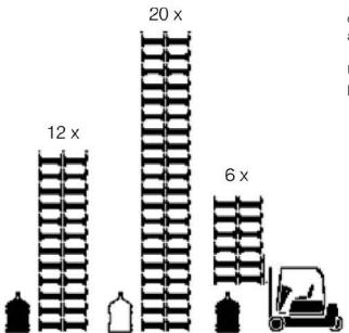
The MODULABLE racks can be stacked on top of each other to form a column of 12 racks with water-filled bottles and up to 20 racks with empty bottles.
